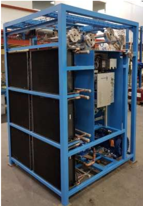
Single-shaft Compressor-Generator-Turbine unit & ancillaries (developed by Enogia SAS)
