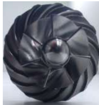
Single-shaft Compressor-Generator-Turbine unit & ancillaries (developed by Enogia SAS)
