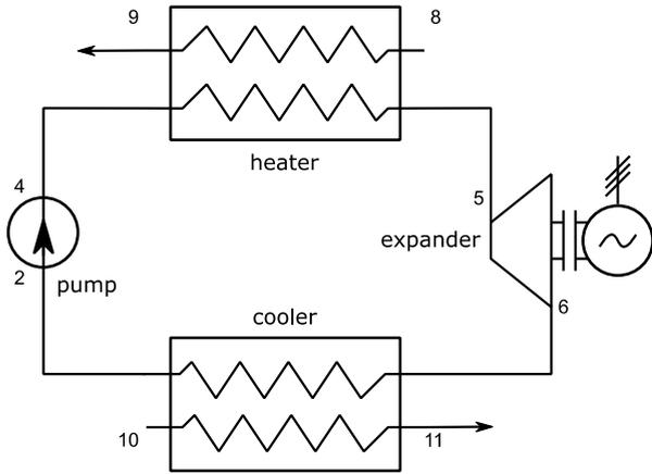
Fig. 1. TFC system components.
