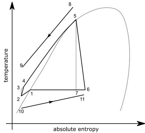
Fig. 2. TFC system temperature-entropy chart.
