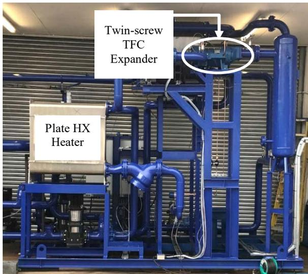
Fig. 5. TFC Pilot Test-rig at Spirax Sarco.
