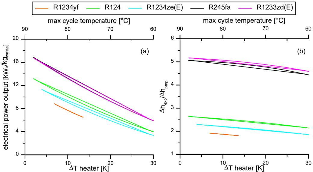
Fig. 3. Theoretical analysis of working fluid performance in a TFC system
