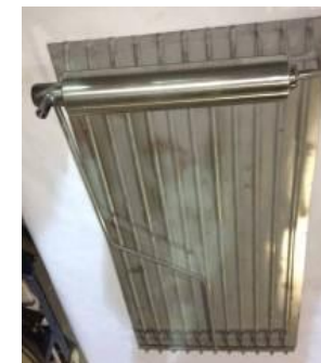
Flat Heat Pipe System
