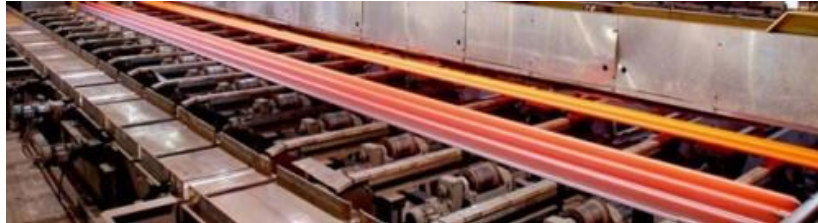
Figure 9: Facility: Rail Mill; Product: Rail; Average T a :around 500°C
