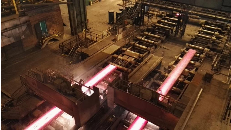
Figure 2: Continuous Casting Zone
