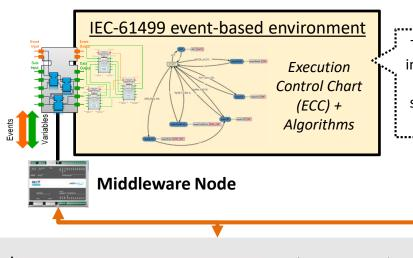
The node is programmed through IEC-61499 to implement a simplified state machine describing the current condition of the mechatronic system. Its evolution is triggered directly by the events generated by the PLC
