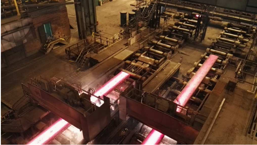
Figure 2: Continuous Casting Zone
